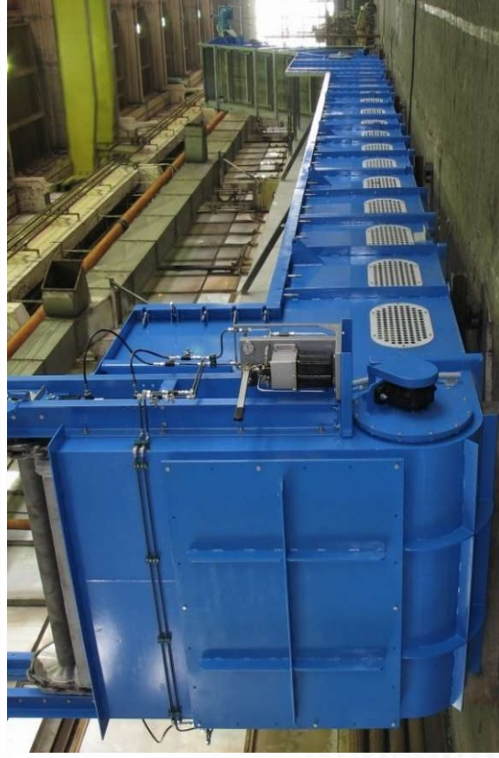
Ash conveyor (l. 21m , h. 5m )
